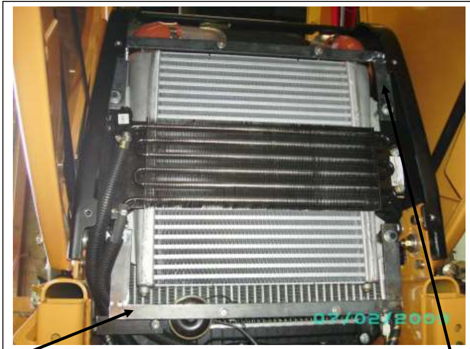
Lower condenser bracket in place
