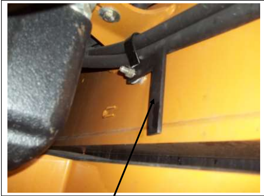
Drier bracket in place.
