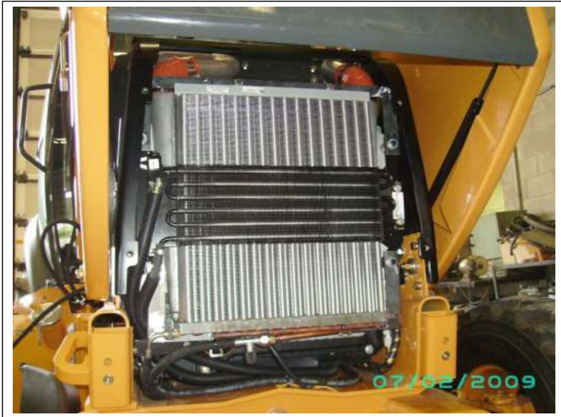
Condenser and hoses in place
