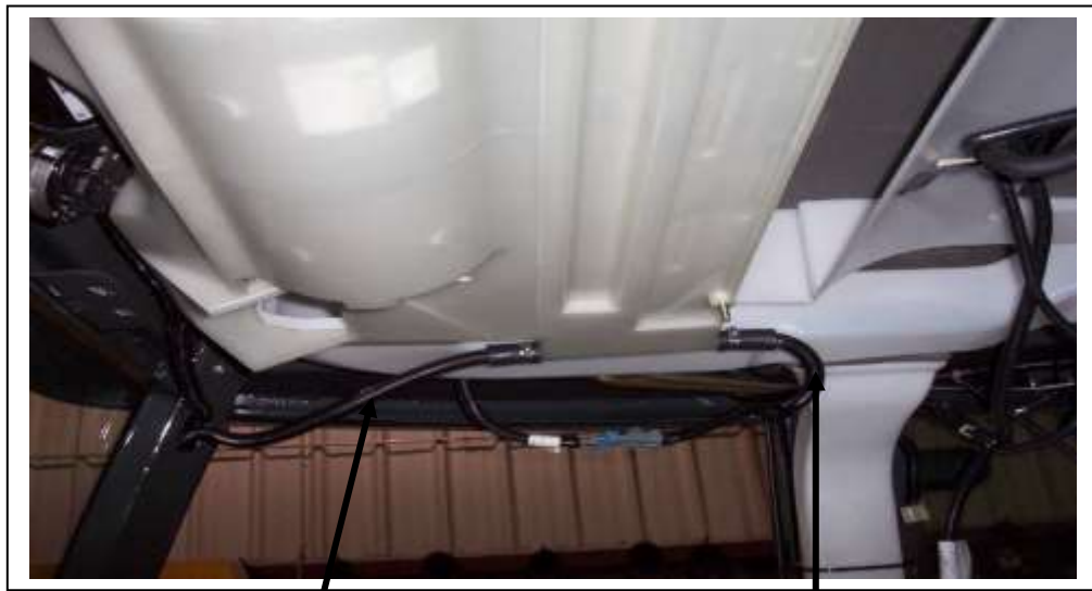
Front right drain tube
